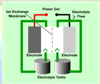
Modern flow cells are generally two electrolyte systems in which they act as liquid energy carriers, are pumped simultaneously through the two half-cells of the reaction cell separated by a membrane.
